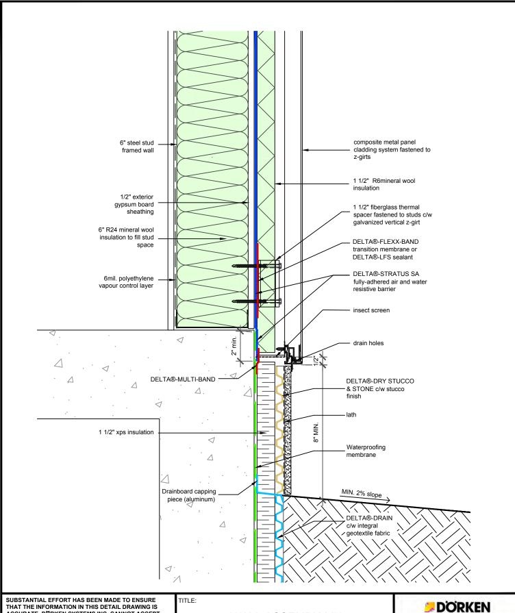
WALL ASSEMBLY #1: TYPICAL BASE OF WALL AT FOUNDATION
