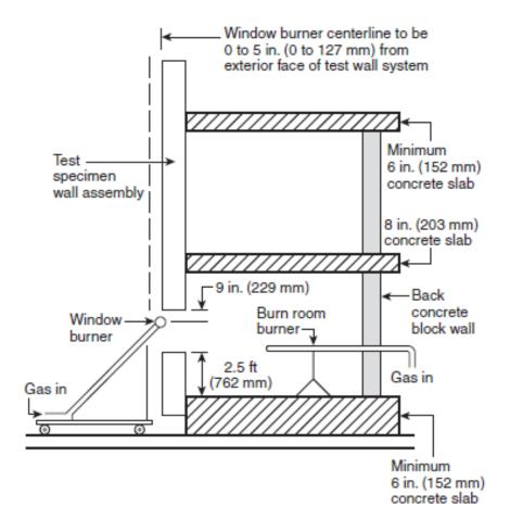
Two burners are ignited to produce a specific time-temperature profile in the room and on the exterior face of the wall.
