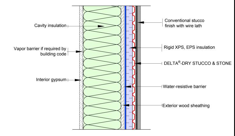
Option 2 Will provide drainage behind stucco only. Does not provide drying for exterior sheathing.
