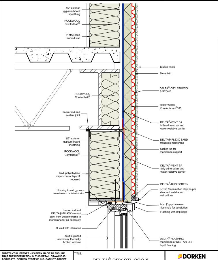
DELTA®-DRY STUCCO & STONE WITH EXTERIOR INSULATION TYPICAL PUNCHED WINDOW HEAD
